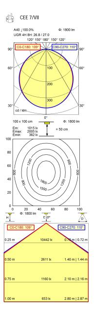
light source LED work equipment electronic transformer connected load 100-240 V, 50/60 Hz; secondary 24 V, DC power consumption env. 38 W luminous flux approx. 2.000 lm luminous efficiency approx. 61 lm/W light type/-color D50 standard light; cold white colour temperatur approx. 5.000 K color rendering index CRI > 95; R9 > 85 light distribution direct
